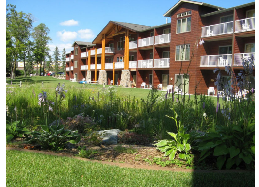
This large rain garden is at The Lodge in Detroit Lakes. It captures some of the water from the building's roof and parking lot and keeps it from going into Big Detroit Lake.
